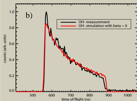
And b) Electron t.o.f. distribution after photodetachment of OH<sup>-</sup>, where the black curve shows the measurement and the red curve the simulation.
