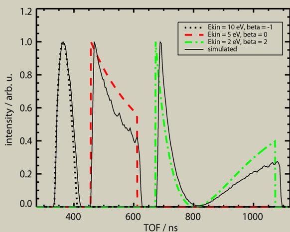
Fig. 3: Electron time of flight distributions for different electron energies and anisotropy parameters calculated using Eq. 3 (dotted lines) and simulated using Simion (solid lines). The kinetic energy of the ions was 4.8 keV.
