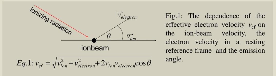
Fig.1: The dependence of the effective electron velocity  $v_{ef}$  on the ion-beam velocity, the electron velocity in a resting reference frame and the emission angle.
